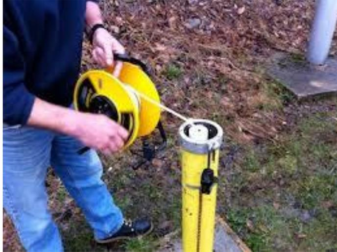
The Geotech ET is a user-friendly device used to measure the depth of groundwater from the surface. Its use in doing so is particularly relevant to the Danda Ecological Monitoring Program because it allows the collection of groundwater level data over time. This data can be used and analyzed to understand how changing water levels affect the environment and ecology of the Danda River as well as the economies of surrounding villages, towns, and municipalities.
